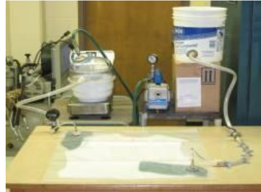
Figure 5. Generation III Assembled. The assembly of the configuration with improvements.
